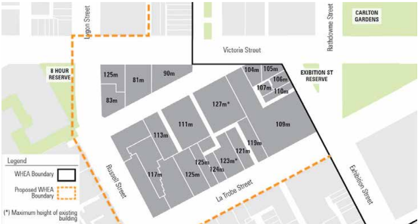
Figure 12 - Recommended DDO for Mixed Use Zone (City of Melbourne): mandatory maximum building height (10m above 'concealment height' when viewed from REB northern forecourt)
